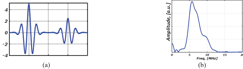
FIGURE 1. Short-duration pulses (a) do not lead to harmonic spacing in frequency domain (b). The second harmonic signal is masked by the fundamental component.
